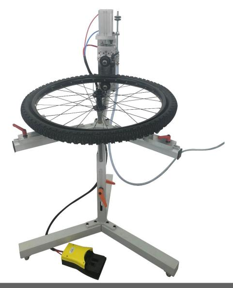
Simple fixture for manual and easy tire fitting
