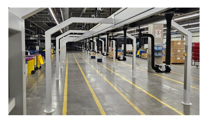
The Smart Aerial Line for bike assembly is a totally innovative overhead conveyor based on modular design. Any length can be proposed, based on 4m long sections providing the smallest footprint for a defined number of working stations and given pitch.
