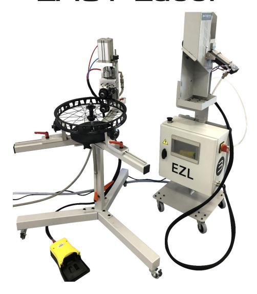
Nipple feeder with electronic control of screwing for balanced and easy lacing of any kind of wheel
